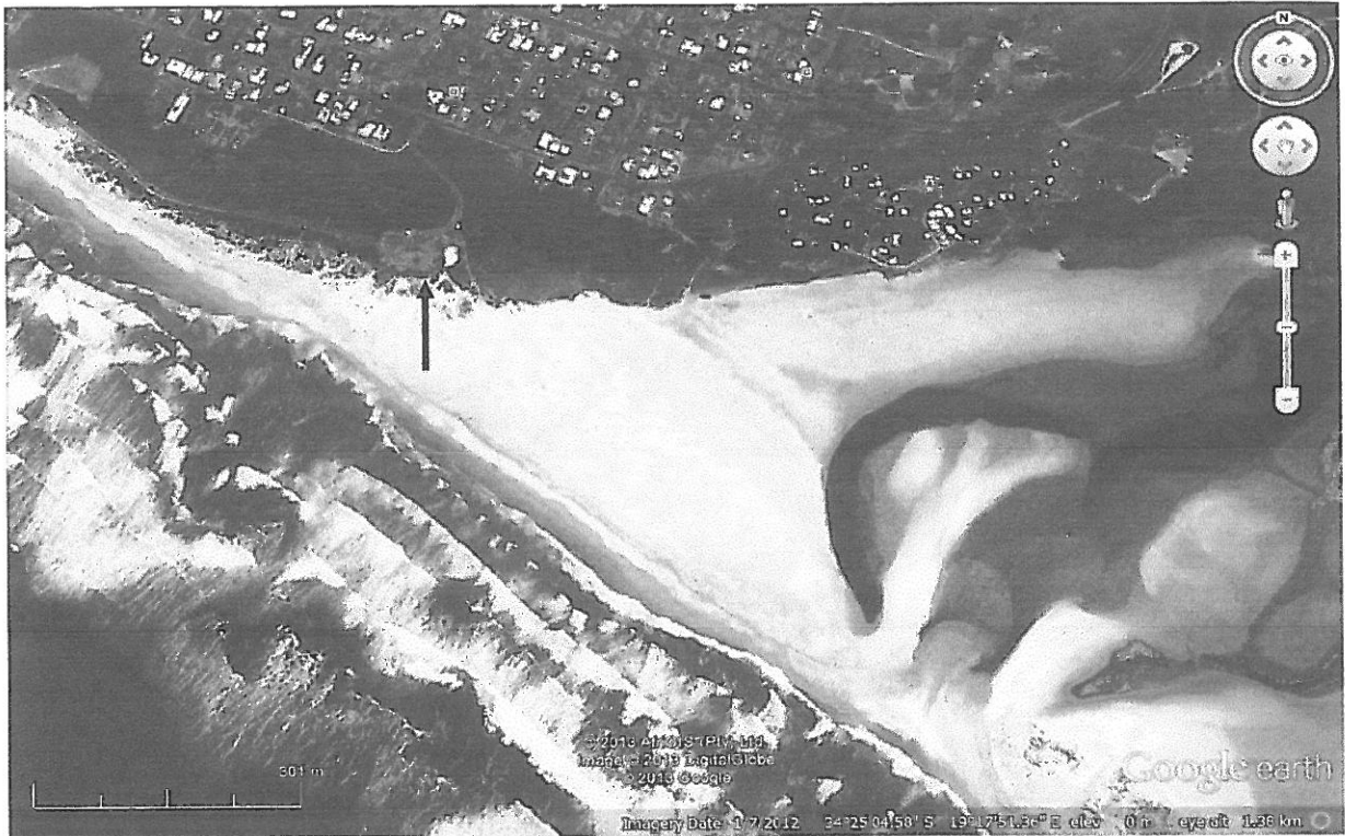
AERIAL PHOTO showing the location of the Grotto Bay parking area (marked with the arrow) where the protection works are to be implemented by means of some form of artificial stabilization of the bank of the parking area. Note the old area where the estuary breached that is now blocked by sand dunes from where sand will be sourced for the protection and to return the breach area to the original.
